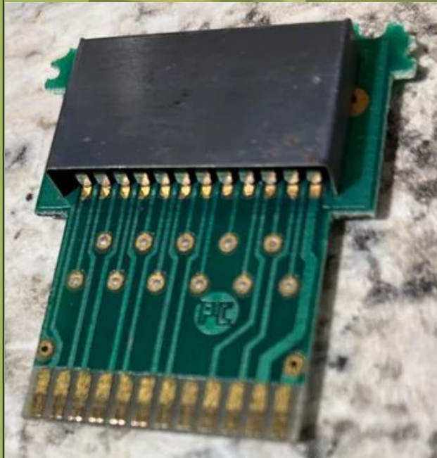
ATARI 2600 BANKSWITCH PCB FRONT
